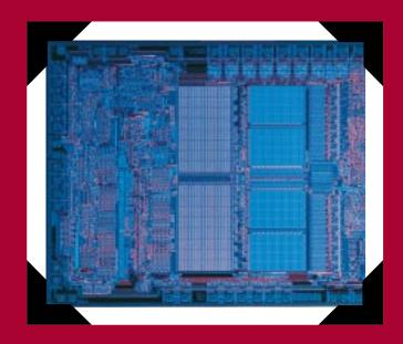
he 68HC11E9 has 12 Kbytes ROM, 512 bytes EEPROM, 512 bytes RAM, SPI, SCI, A/D converter, and 38 I/O pins. The timer system allows 3 or 4 input captures, 4 or 5 output compares, and real-time interrupt.
