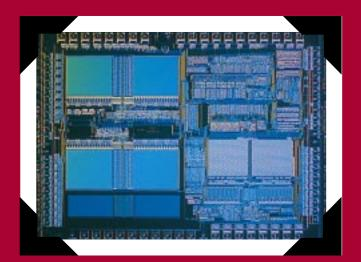
he 68HC711K4 is a high speed, large memory microcontroller with plenty of I/O. It offers 24 Kbytes of EPROM, 640 bytes of EEPROM, 768 bytes of RAM, A/D converter, SPI, SCI and 62 I/O pins. This K-series member offers an address space greater than 1 Mbyte with address expansion lines.
